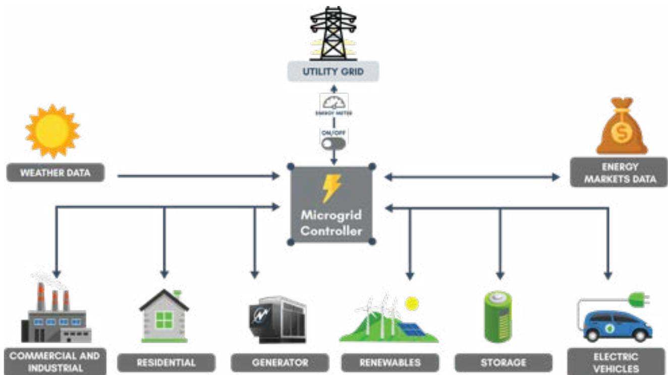
A microgrid must be able to supply energy to its connected loads, independent of the utility, so generation sources must exist within the microgrid. These sources could range from readily controlled to intermittent, to not controllable. This could be renewable (e.g., solar PV, wind, biomass; or solar thermal and hydro) or non-renewable (e.g., diesel, NG, combustion turbines, reciprocating engines, cogeneration, CHP, turbines, microturbines).
