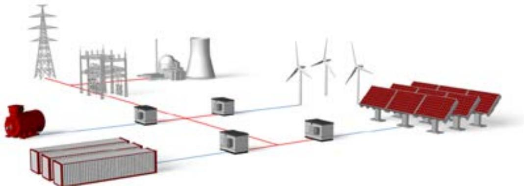
The microgrid controller configures and dispatches the most reliable and economic mix of resources for use at any given time. This might mean integrating on-site renewable energy with other generation resources to overcome the 'variability' of solar and wind—the problem of non-production by these resources when the sun doesn't shine or wind doesn't blow.
